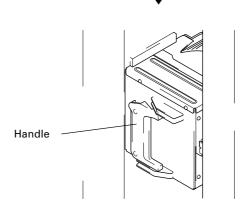
Shown above is the insertion to the front magazine bay. Though the insertion to the rear magazine bay is almost same but note that the proper installation position is in the place where it is very secluded.
